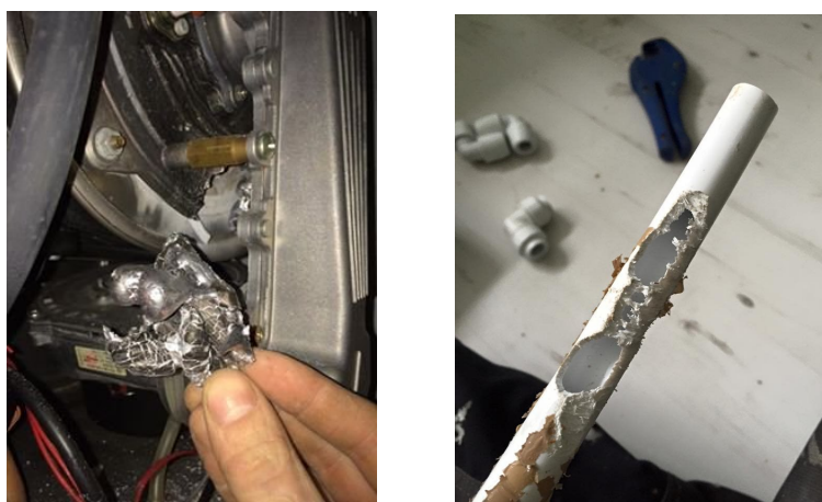
Left: unpredictable boiler fault (Rob Davis) Right: pipe damaged by vermin (Mark Cokayne)
