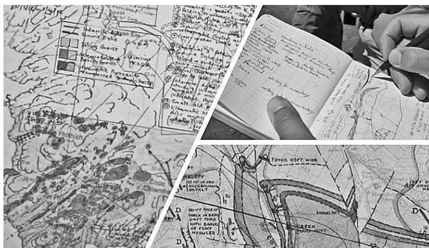
FIGURE 12.4 Geological artefacts created during the making of a geological map. (Left: field slip—a base map on which to make marks, symbols, and notes to represent the geology being observed or inferred. Top right: notebook for recording observations, sketching geological features, and jotting down ideas and interpretations. Bottom right: fair copy map produced from field slips and notebooks after analysing the field work.)
